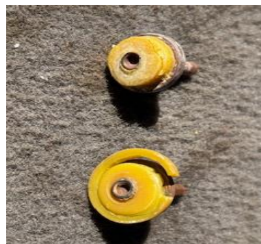
Photo 7 – damaged tap washers.
